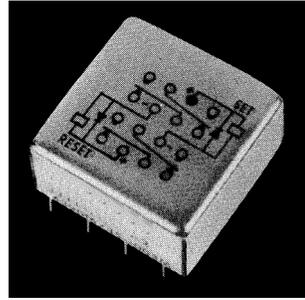
The dual coil version of the 3SBM magnetic latching relay is now available with coil transient suppression with or without blocking diodes for reverse polarity protection. This hybrid magnetic latching relay is an addition to the growing family of .150 grid relays. The diode method is employed to limit the back EMF generated when the coil circuit is opened in order to protect other circuit components such as semiconductors. The contact load
