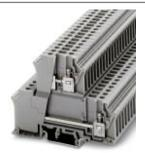
Feed-through terminal block, connection method: Screw connection, cross section: 0.2 mm<sup>2</sup> - 4 mm<sup>2</sup>, AWG: 24 - 12, width: 6.2 mm, color: gray, mounting type: NS 35/7,5, NS 35/15, NS 32
