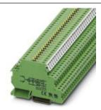
Relay terminal block, with soldered-in miniature relays, contact (AgNi+Au): small to medium loads, 1 N/O contact, input voltage 24 V AC/DC, with integrated "manual", "0", "automatic" switch, for assembly on NS 35/7.5, terminal width 6.2 mm
