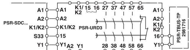
Figure 7 Wiring via T-BUS DIN rail connector
