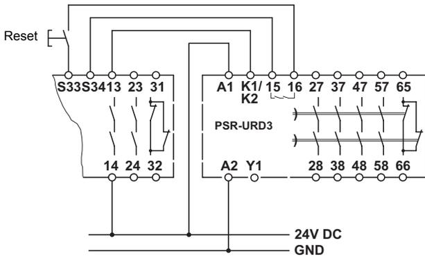
Figure 6 Wiring via connection terminal blocks
