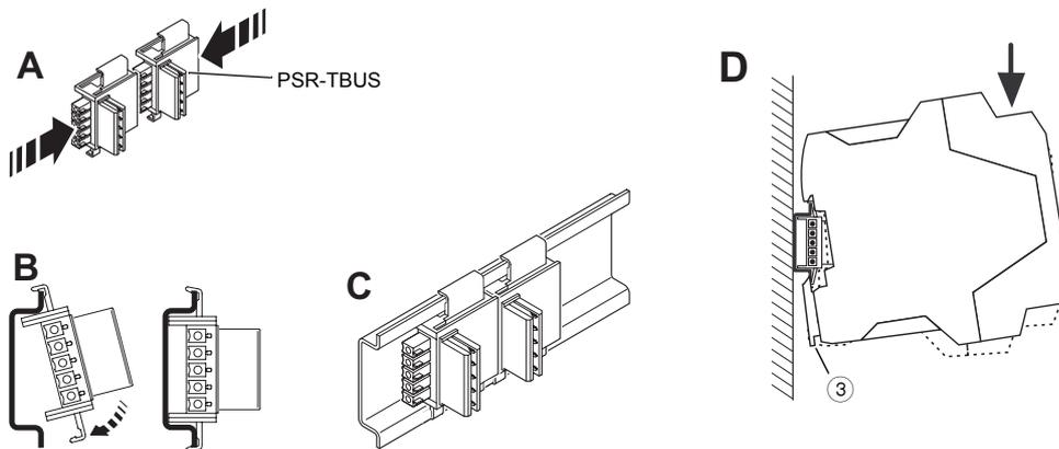
Figure 3 Using the T-BUS DIN rail connector
