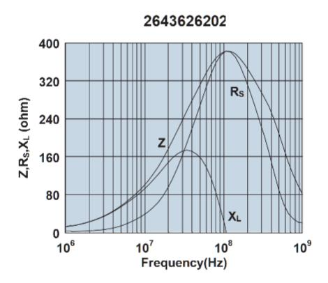
Impedance, reactance, and resistance vs. frequency.
