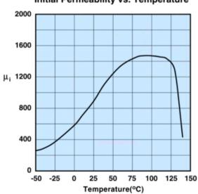
Measured on a 17/10/6mm toroid at 100kHz.
