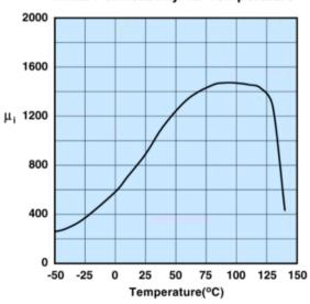
Measured on a 17/10/6mm toroid at 100kHz.
