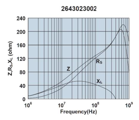
Impedance, reactance, and resistance vs. frequency.
