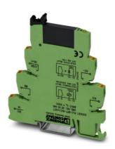
PLC actuator interface, consisting of PLC-BPT...ACT basic terminal block with Push-in connection and plug-in miniature solid-state relay, for mounting on NS 35/7,5 DIN rail, input: 24 V DC, output: 3 - 33 V DC/3 A
