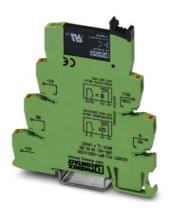
PLC sensor interface, consisting of PLC-BPT...SEN basic terminal block with Push-in connection and plug-in miniature solid-state relay, for mounting on NS 35/7,5 DIN rail, input: 24 V DC, output: 3 - 48 V DC/100 mA
