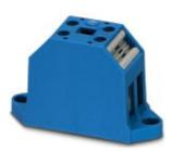
Device terminal block, Connection method: Screw connection, Number of positions: 1, Cross section: 0.5 mm<sup>2</sup> - 16 mm<sup>2</sup>, AWG: 20 - 6, Width: 24.8 mm, Height: 40 mm, Color: blue, Mounting type: Screw mounting
