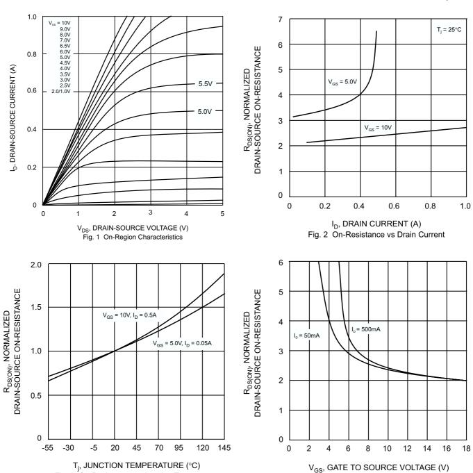
Fig. 3 On-Resistance vs Junction Temperature
