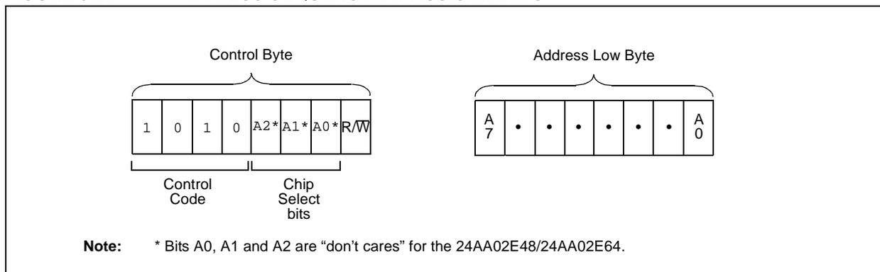
FIGURE 5-1: CONTROL BYTE ALLOCATION
