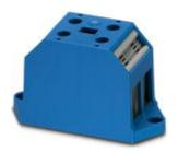
Device terminal block, Connection method: Screw connection, Number of positions: 1, Cross section: 0.75 mm² - 35 mm², AWG: 18 - 2, Width: 34.8 mm, Height: 44.9 mm, Color: blue, Mounting type: Screw mounting
