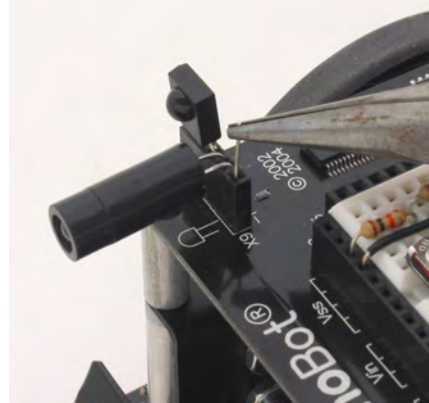
Figure 3-4 Clip Leads from Spare Components and Insert them into Loose Header Sockets
