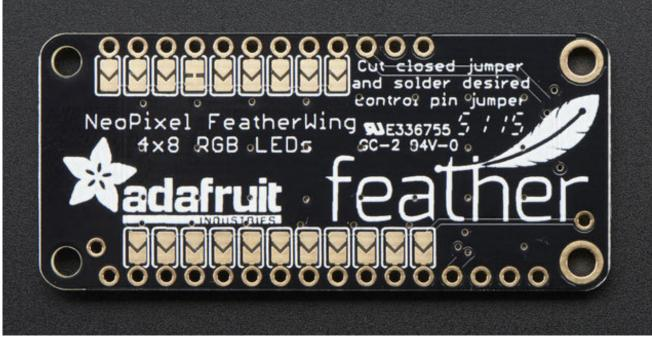
On the bottom, we have a range of pins that are available for use as the 'control pin'
