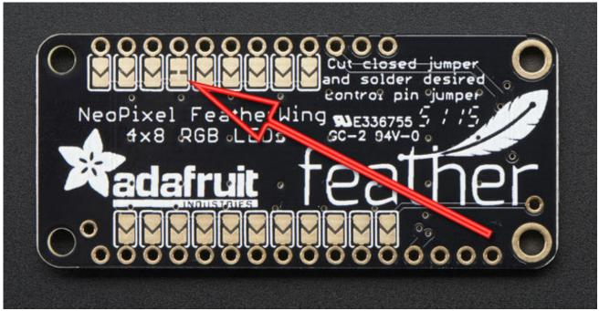
This pin is **#6** for Feather 32u4 and M0s, and is **#16** on ESP8266 Feather.
