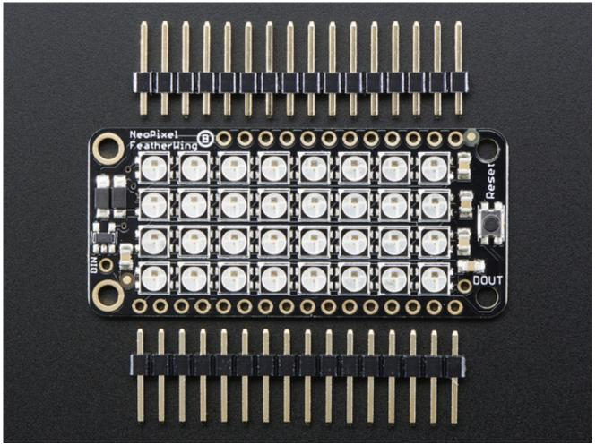
A level-up shifter converts the 3.3V logic of the Feather to the power line voltage. If, say, you need MORE blinky, you can chain these together. For the second Wing, connect the DIN connection to the first Wing's DOUT. Also connect a ground pin together and power with an independant 5V supply to keep from loading the power supply too much.
