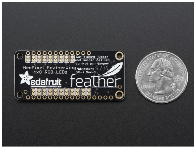
To make it easy to start, the LEDs are by default powered from *either* the USB power line or Battery power line, whichever is higher. Two Schottky diodes are used to switch between the two. This power arrangement is able to handle 1 Amp of constant current draw and maybe 2A peak, so not a good way to make a flashlight. It's better for colorful effects.
