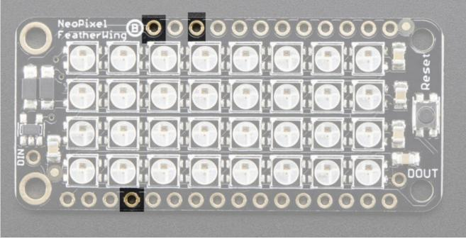
The bottom ground pin is also used of course, for both power and data ground reference.
