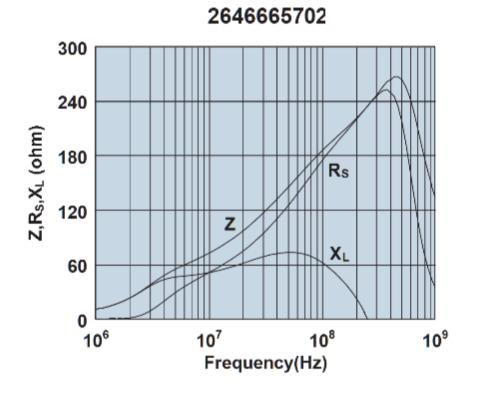
Impedance, reactance, and resistance vs. frequency.
