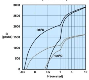
Measured on a 17/10/6mm toroid at 10kHz.
