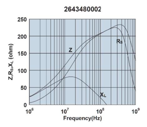
Impedance, reactance, and resistance vs. frequency.
