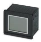
Touch panel with 7.1 cm/2.8" TFT-Display (Analog resistive (polyester)), 320 x 240 Pixel (QVGA), 4 colors, Cortex™-M3 120 MHz, without, 1 x Ethernet (10/100 Mbps), RJ45, Keil RTX (RTOS) and User software: PC Worx. (Bus system: without)
