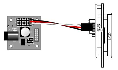
Serial devices can communicate directly with the BASIC Stamp on headers A2, A3, P8, and P9. They can communicate with the AVR on headers A0, A1, A2, and A3, but to do so requires the appropriate AVR firmware to be loaded.
