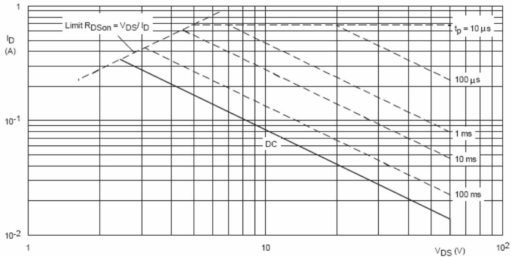
T<sub>sp</sub> = 25 °C; I<sub>DM</sub> is single pulse; V<sub>GS</sub> = 10 V
