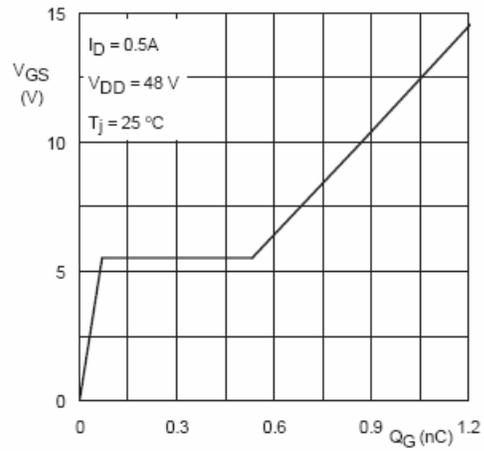
$I_D = 0.5\text{ A}$ ;  $V_{DD} = 48\text{ V}$
