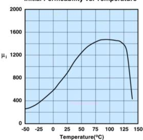
Measured on a 17/10/6mm toroid at 100kHz.
