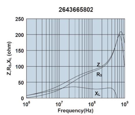
Impedance, reactance, and resistance vs. frequency.
