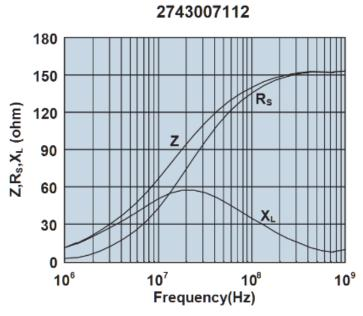
Impedance, reactance, and resistance vs. frequency.
