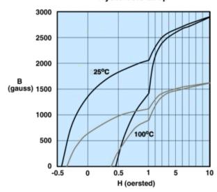
Measured on a 17/10/6mm toroid at 10kHz.
