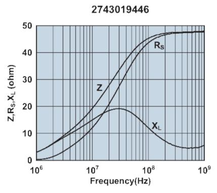
Impedance, reactance, and resistance vs. frequency.
