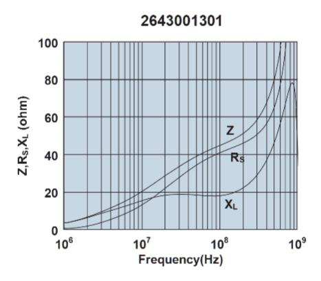
Impedance, reactance, and resistance vs. frequency.
