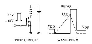
$$\begin{array}{ll} \text{Peak I}_{AR} = 15\text{A, R}_{G} = 25\Omega & \text{E}_{AS} = \frac{1}{2} \cdot \text{L} \cdot \text{I}^{2} \cdot (\frac{\text{BVDSS}}{\text{BVDSS-V}_{DD}}) \end{array}$$
