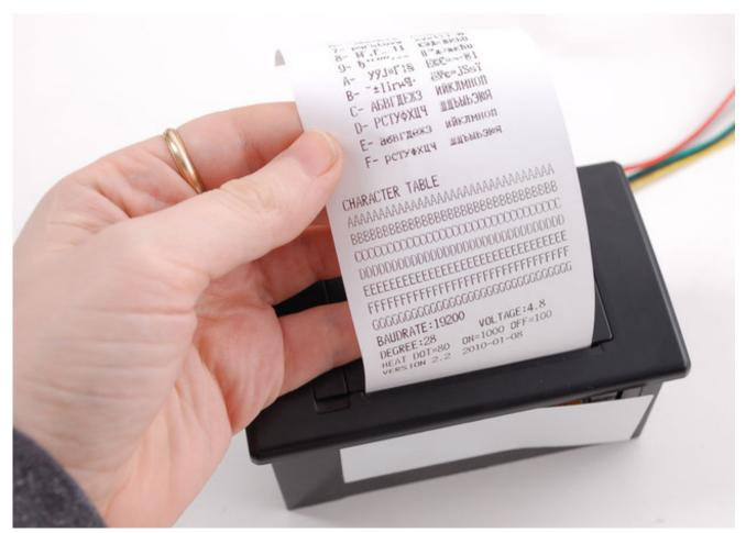
If you don't get a printout, check that the paper is inserted correctly and not binding, that the power is correctly wired, power supply is plugged in, etc. Then try again, holding down the button when connecting power.
