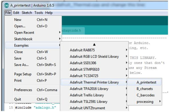
If your printer test page shows 'BAUDRATE: 9600', you'll need to make a small change to the library source code. Using a text editor (Notepad, etc.) open the file Adafruit\_Thermal.cpp and change this line:
