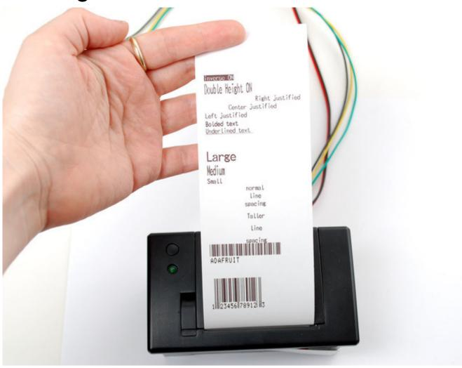
The thermal printer has a few handy things it can do, most of which are in the **A\_printertest** sketch. These are shown in the image above. In order, starting from the top:
