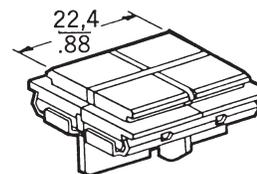
Silicone rubber baffles prevent light spillage from one section to another. Screen caps and legend inserts are transparent colorless. Bases are translucent colored.
