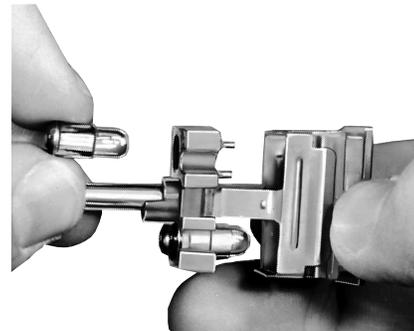
**Without tool.** Remove display screen/lampholder assembly from 2C200 operator-indicator (or 2F200 indicator). Unit is keyed to maintain proper orientation when replacing. Use only flange base T-1 $\frac{3}{4}$  lamps with 2C200 and 2F200 devices.
