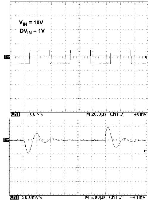
FIGURE 52. LINE TRANSIENT RESPONSE, 0.001  $\mu F$  LOAD CAPACITANCE
