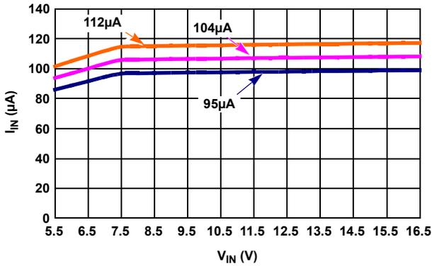
FIGURE 44.  $I_{IN}$  vs  $V_{IN}$ , 3 UNITS
