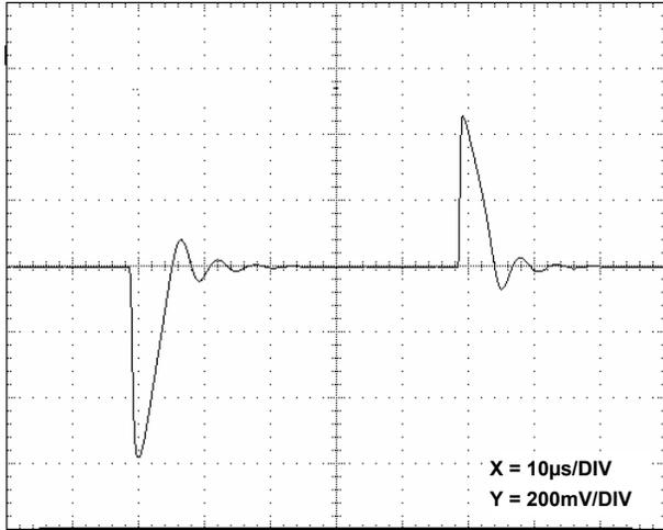
FIGURE 38. LINE TRANSIENT RESPONSE, 0.001µF LOAD CAPACITANCE
