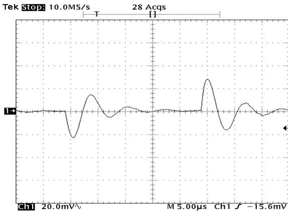
FIGURE 24. LINE TRANSIENT RESPONSE, 0.001 $\mu$ F LOAD CAPACITANCE
