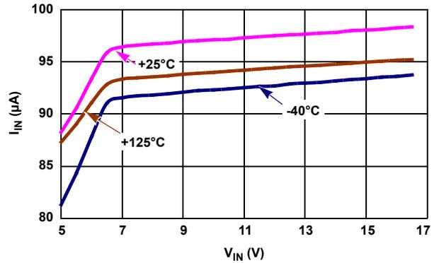
FIGURE 3.  $I_{IN}$  vs  $V_{IN}$ , 3 TEMPERATURES
