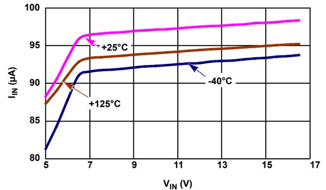
FIGURE 31.  $I_{IN}$  vs  $V_{IN}$ , 3 TEMPERATURES
