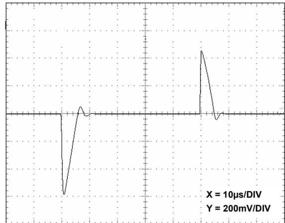
FIGURE 37. LINE TRANSIENT RESPONSE, NO CAPACITIVE LOAD
