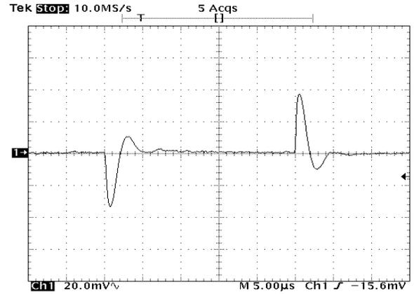
FIGURE 23. LINE TRANSIENT RESPONSE, NO CAPACITIVE LOAD
