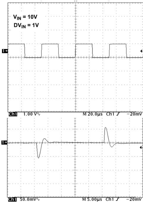
FIGURE 51. LINE TRANSIENT RESPONSE, NO CAPACITIVE LOAD
