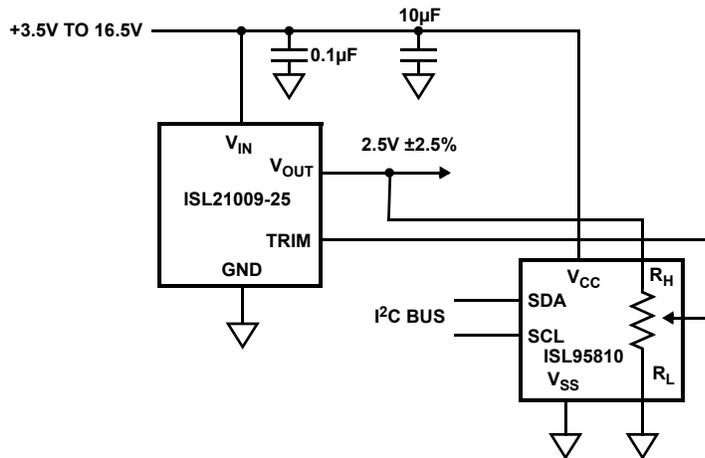
FIGURE 62. OUTPUT ADJUSTMENT USING THE TRIM PIN
