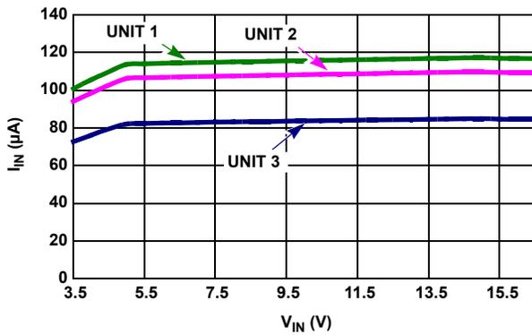
FIGURE 16.  $I_{IN}$  vs  $V_{IN}$ , 3 UNITS
