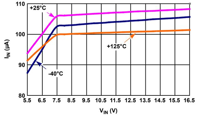
FIGURE 45.  $I_{IN}$  vs  $V_{IN}$ , 3 TEMPERATURES
