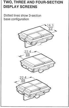
Silicone rubber baffles prevent light spillage from one section to another. Screen caps and legend inserts are transparent colorless. Bases are translucent colored.
