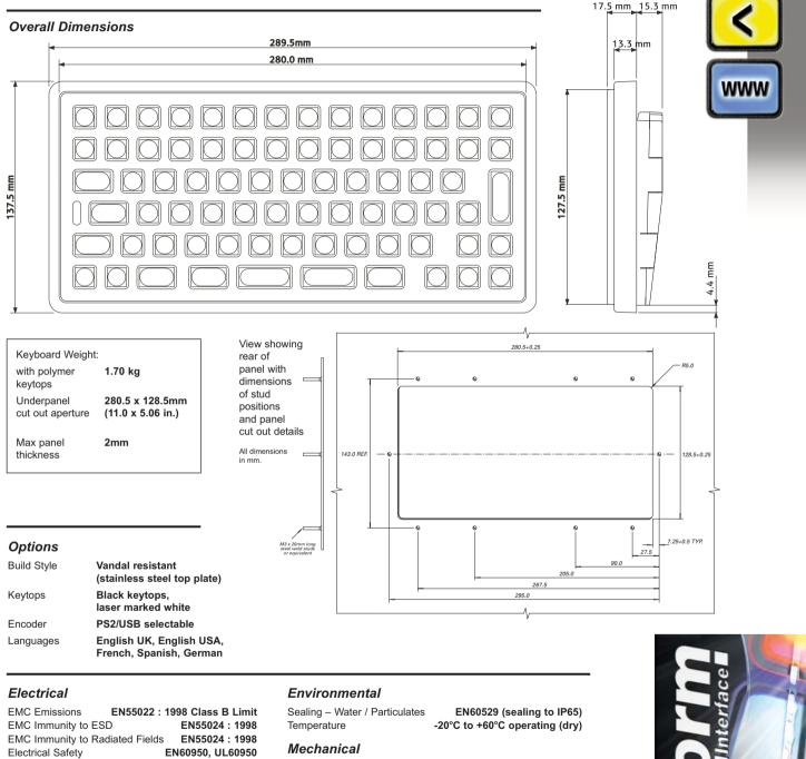
or USB Interface Supply requirements voltage +5V nominal (5.5V to 4.75V) Supply requirements
