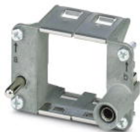
Module carrier frame, Size: B6, Type: for the panel mounting side (a, b, c, ...), Connection cross section: 4 mm² ... 6 mm², Application: Module carrier frame
