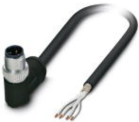
Sensor/Actuator cable, 4-position, RADOX® GKW S halogen-free, black, shielded, Plug angled M12 SPEEDCON, A-coded, on free cable end, Cable length: 5 m, For railway applications
