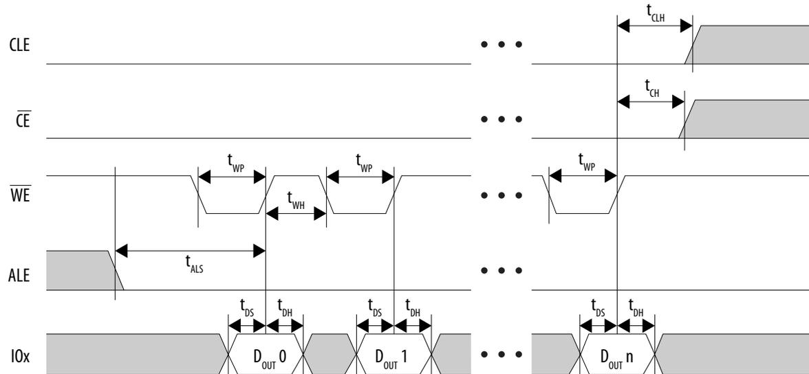
Figure 21. NAND Data Input Cycle Timing Diagram
