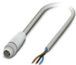
Sensor/Actuator cable, 3-position, PP-EPDM halogen-free, Gray RAL 7035, Plug straight M8, on free cable end, Cable length: 5 m, Hygienic design, with plastic knurl
