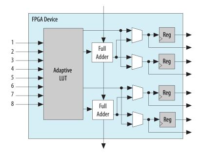
The Quartus Prime software optimizes your design according to the ALM logic structure and automatically maps legacy designs into the Arria 10 ALM architecture.
