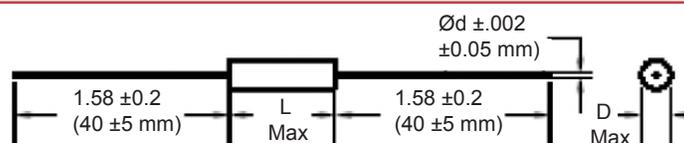
Lead Material: tinned copper wire
