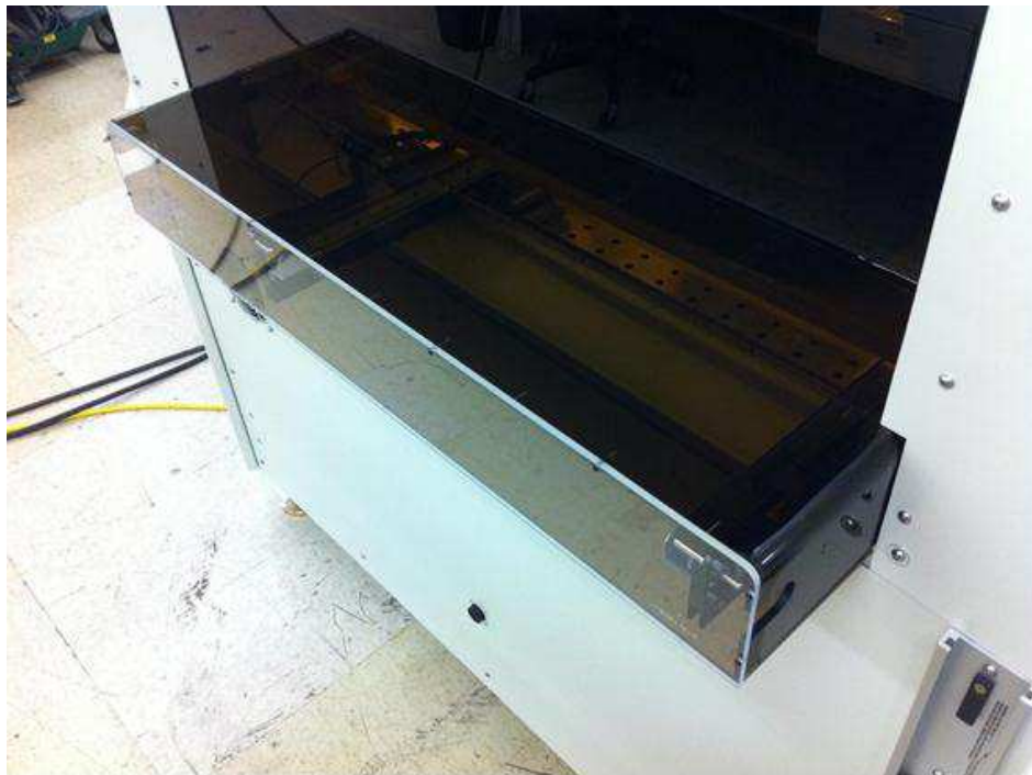
Infeed Conveyor with Block-Off Plate for Stand Alone (Reverse Shuttle) Operation
