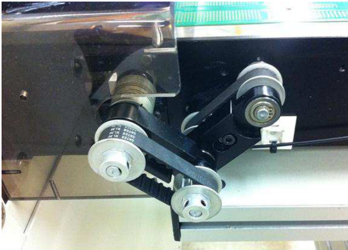
Conveyor Extension Drive Coupling
