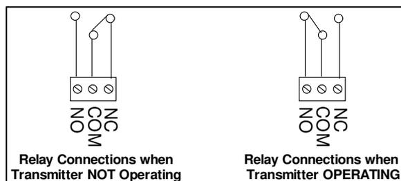
Relay output '1' provides a longer momentary output (approx 1/2 second) this may be removed (see below). For solenoid driven traps.
