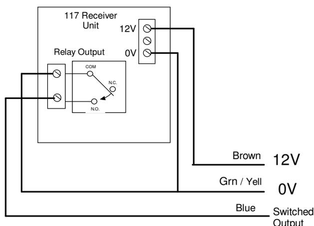
7. When operated, the receiver provides an output (Blue Wire) which momentarily connects to 0V.
