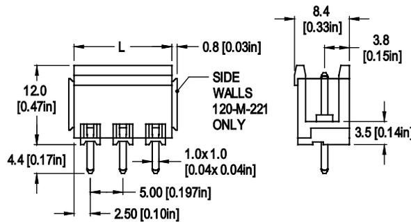
Dimensions: mm (in.) When locating connector, allow 0.5 mm clearance around it for process-induced variations. Length of Connector (L) L = No. of Poles x Center to Center Spacing: - 1.8 mm
