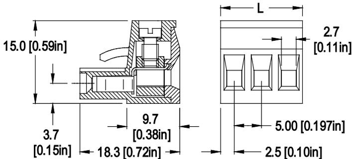
Dimensions: mm (in.) When locating connector, allow 0.5 mm clearance around it for process-induced variations. Length of Connector (L) L = No. of Poles x Center to Center Spacing
