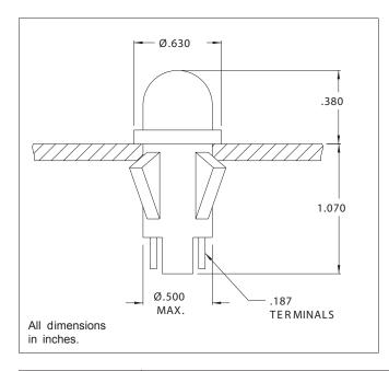
Solid-state indicator lights complete with built-in current-limiting resistor and rectifier diode.
