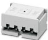
Plug component, Nominal current: 10 A, Rated voltage (III/2): 24 V, Number of positions: 4, Pitch: 2.4 mm, Color: white, Contact surface: Tin, Mounting: Direct plug-in method, for flexible PCBs with a width of 10 mm and a permissible PCB thickness in the contact zone of 0.15 mm ... 0.3 mm
