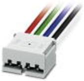
Plug component, Nominal current: 10 A, Rated voltage (III/2): 24 V, Number of positions: 4, Pitch: 2.4 mm, Color: white, Contact surface: Tin, Mounting: Direct plug-in method, Length of the punched-on cables: 500 mm, for flexible PCBs with a width of 10 mm and a permissible PCB thickness in the contact zone of 0.15 mm ... 0.3 mm
