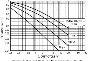
Figure 7. Typical Derating Factor for Duty Cycle
