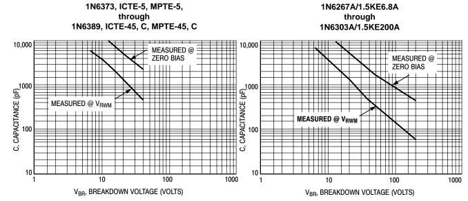
Figure 3. Capacitance versus Breakdown Voltage
