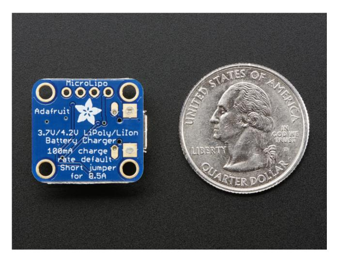
Adafruit has a few small basic chargers that can satisfy your LiPo charging needs. **All of these chargers can only do 1-cell chargers for 3.7V/4.2V cells.** These are by far the most common and all the Lilon/LiPo batteries in the Adafruit shop will work quite nicely.
