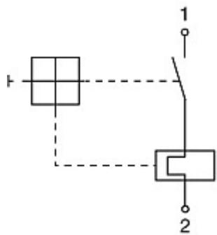
Miniaturised single pole thermal circuit breaker with push-to-reset tease free, trip-free, snap action mechanism (R-type TO CBE to EN 60934), threadneck mounting.
