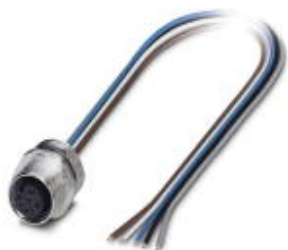
Sensor/actuator flush-type socket, 5-pos., M12, A-coded, front/screw mounting with Pg9 thread, with 0.2 m TPE litz wire, 5 x 0.34 mm 2
