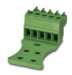
Plug component, Nominal current: 8 A, Rated voltage (III/2): 160 V, Number of positions: 5, Pitch: 3.5 mm, Connection method: Screw connection with tension sleeve, Color: green, Contact surface: Tin
