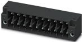
The figure shows a 10-pos. version with 20 contacts
