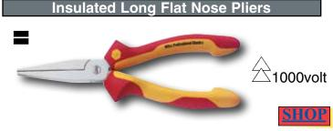
328 Long Nose Pliers With Cutters. Insulation According to VDE 0682/part 201, EN/IEC 60900, ASTM F-1505-01, NFPA70E & CSA,  $\bigwedge$  up to 1000 Volt. Individually Tested. Drop-forged from C70 special tool steel, cutters additionally induction hardened to approx. 64HRC, chrome-nickel plated, mirror-polished, ergonomic comfort grip with slip guard, half-round jaws, serrated gripping surface.
