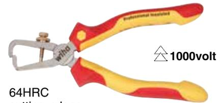
**32860 Stripping Pliers. Insulation According to VDE 0682/part 201, EN/IEC 60900, ASTM F-1505-10, NFPA70E and CSA, up to 1000 Volt. Individually Tested.** Heavy duty forged with induction hardened cutting edges for even stripping of insulation. Drop-forged from special tool steel, chrome & nickel plated, mirror-polished. Ergo comfort grip with slip guard. Spring & adjusting screw, for stripping up to #8 AWG.
