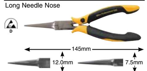
**32746 ESD Safe Pliers, Long Needle Nose Pliers, Straight, Serrated Jaws** Pliers drop-forged for an ideal material structure. Precisely aligned, jaws, hardened. ESD Safe Dissipative.
