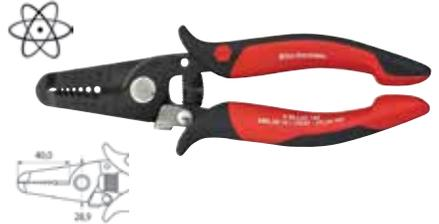
**56871 Stripping Pliers** Wide long head with ridged gripping surface, shears blade and firm wire stripping stations. With opening spring and locking mechanism. Wire stripping stations 0.81 / 1.0 / 1.3 / 1.6 / 2.0 / 2.59mm, AWG 20 / 18 / 16 / 14 / 12 / 10.
