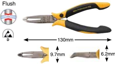
**32728 Oblique Front Cutters, Very Small Head, 40°, Flush** Oblique Cutters drop-forged for an ideal material structure. Precise aligned cutting edges are additionally induction hardened at a hardness of Approx. 64°HRC. ESD Safe Dissipative.
