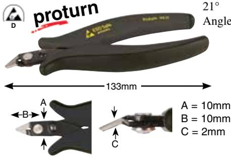
**45823 Protturn ESD Safe 21° Precision Cutters/Flush Cut** ESD standard IEC 61340-5-1. C70 special tool steel. Glare free, black finish. ESD Safe handle with non-slip grips.
