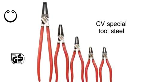
**32627 5 Piece 90° Angle Internal Ring Pliers Set** Shape D, 90° angled tips. Die forged cylindrical precision formed. CV Special tool steel. For inserting & removing internal retaining rings. Soft vinyl grips.
