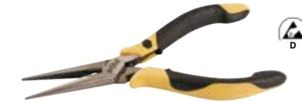
**32762 ESD Safe Long Nose Pliers With Return Spring** Extra long cutters for flat and round cables. Serrated jaws. Long life edge is achieved through additional induction hardening to approx. 64HRC. Special C70 tool steel forgings. Two component non-slip soft grip handle, ESD Safe Dissipative.
