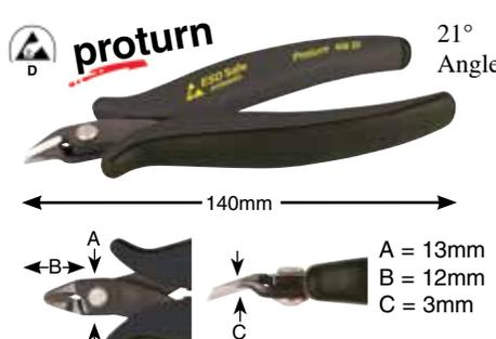
**45822 Protturn ESD Safe 21° Precision Cutters/Flush Cut** ESD standard IEC 61340-5-1. C70 special tool steel. Glare free, black finish. ESD Safe handle with non-slip grips.
