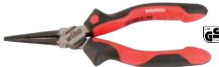
**30921 Industrial Long Round Nose Pliers** DIN ISO 5745 Extra long head. Gripping surfaces serrated and induction hardened. C70 Special tool steel. Two component SoftGrip handle. Gripping and bending of wires and sheet metal parts.
