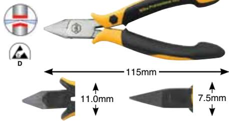
**32710 Precision Cutters, Wide Tapered Head, Full Flush** Cutters drop-forged for an ideal material structure. Precise aligned cutting edges are additionally induction hardened at a hardness of Approx. 64°HRC. Two component non-slip soft grip handle, ESD Safe Dissipative.
