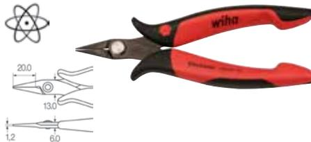
**56801 Electronic Short Nose Precision Pliers** Narrow, short head. Smooth jaws. Width at tip is only 1.2mm. C70 special tool steel. For holding small components as well as for holding and angling wires.
