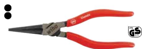
**32633 Long Round Nose Pliers** DIN ISO 5745 Extra long head. Serrated Jaws are induction hardened. Special C70 tool steel forgings. Use for gripping and uniform round bending of wires and sheet metal parts. Soft vinyl grips are oil & solvent resistant.
