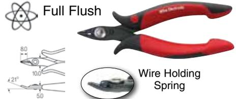
**56813 Precision Electronic Diagonal Full Flush Cutters With Wire Trapping Spring** Extra narrow, short head for working in particularly restricted spaces. Cutting edge - full flush. With return spring. C70 special tool steel. For absolutely flush cutting of copper wires in difficult to access locations.
