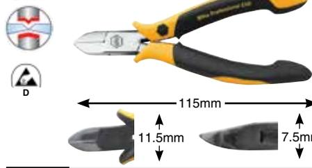
**32716 Precision Cutters, Wide Oval Head, Bevel** Cutters drop-forged for an ideal material structure. Precise aligned cutting edges are additionally induction hardened at a hardness of Approx. 64°HRC. Two component non-slip soft grip handle, ESD Safe Dissipative.
