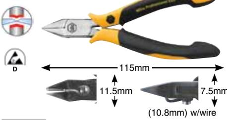
**32711 Precision Cutters, Wide Tapered Head With Wire Trapping Device, Flush** Cutters drop-forged for an ideal material structure. Precise aligned cutting edges are additionally induction hardened at a hardness of Approx. 64°HRC. ESD Safe Dissipative.
