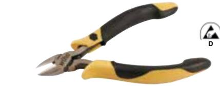
**32760 ESD Safe Precision Flush Cutting Diagonal Cutters** Low wear lap joint, riveted and able to withstand high levels of load. Lightweight action, clean cutting. Long life edge is achieved through additional induction hardening to approx. 64HRC. Special C70 tool steel. Two component non-slip soft grip handle, ESD Safe Dissipative.
