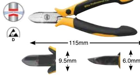
**32714 Precision Cutters, Slim Oval Head, Full Flush** Cutters drop-forged for an ideal material structure. Precise aligned cutting edges are additionally induction hardened at a hardness of Approx. 64°HRC. Two component non-slip soft grip handle, ESD Safe Dissipative.
