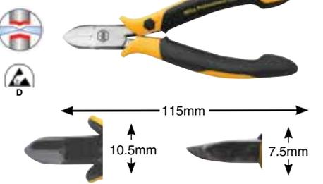
**32712 Precision Cutters, Slim Oval Head, Flush** Cutters drop-forged for an ideal material structure. Precise aligned cutting edges are additionally induction hardened at a hardness of Approx. 64°HRC. Two component non-slip soft grip handle, ESD Safe Dissipative.
