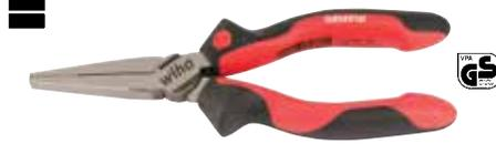
**30919 Industrial Long Flat Nose Pliers** DIN ISO 5745 Extra long head. Gripping surfaces serrated and induction hardened. C70 Special tool steel. Two component SoftGrip handle. Gripping and right-angled bending of wires and sheet metal parts.
