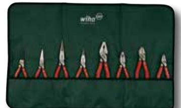
**32608 8 Pc. Pliers/Cutters** Jaws & cutters induction hardened. Long life edge is achieved through additional induction hardening to approx. 60 HRC.
