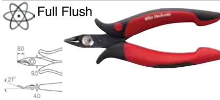
**56812 Precision Electronic Diagonal Cutters, Narrow Shape** Extra narrow, short head for working in particularly restricted spaces. Cutting edge - full flush. With return spring. C70 special tool steel. For absolutely flush cutting of copper wires in difficult to access locations.
