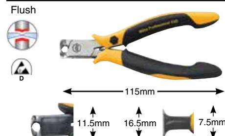
**32734 End Cutters, Wide Head, Flush** End Cutters drop-forged for an ideal material structure. Precise aligned cutting edges are additionally induction hardened at a hardness of Approx. 64°HRC. ESD Safe Dissipative.
