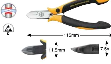
**32720 Precision Cutters, Wide Oval Head, Flush** Cutters drop-forged for an ideal material structure. Precise aligned cutting edges are additionally induction hardened at a hardness of Approx. 64°HRC. Two component non-slip soft grip handle, ESD Safe Dissipative.
