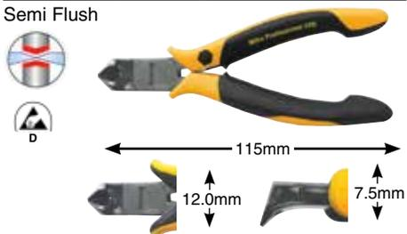
**32726 Oblique Angled Cutters, 29°, Short Head, Semi Flush** Oblique Cutters drop-forged for an ideal material structure. Precise aligned cutting edges are additionally induction hardened at a hardness of Approx. 64°HRC. Two component non-slip soft grip handle, ESD Safe Dissipative.
