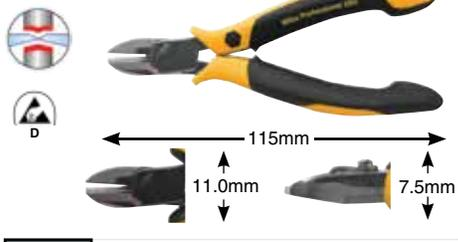
**32721 Precision Cutters, Wide Oval Head With Wire Trapping Device, Flush** Cutters drop-forged for an ideal material structure. Precise aligned cutting edges are additionally induction hardened at a hardness of Approx. 64°HRC. Two component non-slip soft grip handle, ESD Safe Dissipative.
