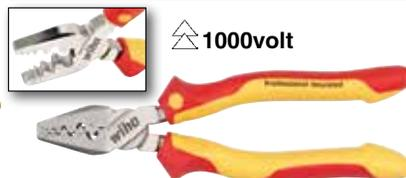
**32841 Insulated Crimping Pliers. Insulation According to VDE 0682/part 201, EN/IEC 60900, ASTM F-1505-10, NFPA70E & CSA, up to 1000 Volt. Individually Tested.** Semi-circular profiles for secure connection between & sleeve and conductor. Long life is achieved through additional induction hardening to 64HRC. C70 special tool steel.
