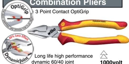
**32820 High Leverage Combination Pliers. Insulation According to EN/IEC, ASTM, NFPA & CSA, up to 1000 Volt. Extra long cutting edge for flat & round cables. Cutting edges additionally induction hardened to approx. 64HRC. C70 Special tool steel. Use for gripping, pulling & holding as well as cutting wires & cables ranging in hardness from soft to extremely hard.**
