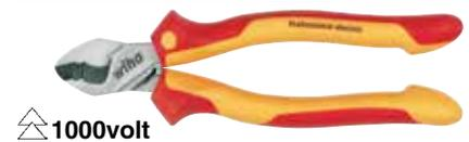
**328 Serrated Edge Cable Cutters. Insulation According to VDE 0682/part 201, EN/IEC 60900, ASTM F-1505-10, NFPA70E and CSA, up to 1000 Volt. Individually Tested.** Light, clean cutting ground precision cutting edges. Durable cutting is achieved through additional inductive hardening to approx. 64HRC. Special tool steel. For cutting of copper & aluminum cables without crushing.
