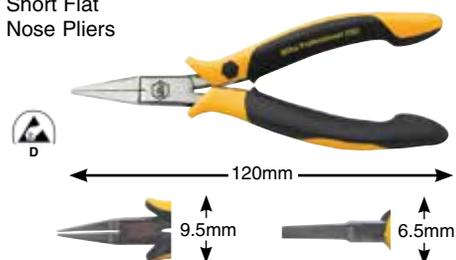
**32752 ESD Safe Pliers, Short Flat Nose Pliers, Smooth Jaws** Pliers drop-forged for an ideal material structure. Precisely aligned, jaws, hardened. Two component non-slip soft grip handle, ESD Safe Dissipative.
