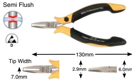
**32732 End Cutters, Extra Slim, Semi Flush** End Cutters drop-forged for an ideal material structure. Precise aligned cutting edges are additionally induction hardened at a hardness of Approx. 64°HRC. ESD Safe Dissipative.
