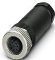
Connector, 8-position, Socket straight M12, A-coded, Screw connection, Knurl material: Zinc die-cast, nickel-plated, Cable gland Pg11, External cable diameter 8 mm ... 10 mm
