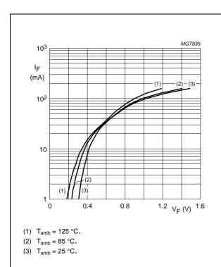
Fig.6 Forward current as a function of forward voltage; typical values.
