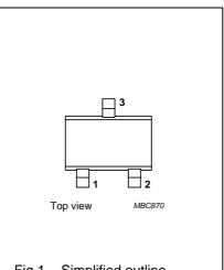
Fig.1 Simplified outline (SOT323; SC-70) and pin configuration.
